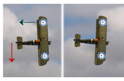
Adverse yaw occurs because a downward deflected aileron causes more drag then the upward deflected aileron. This drag force drifts the airplane out of its flight path during rolls sequences, in a direction opposite to the rolling versus
